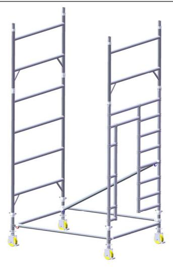
**4** Fit two horizontal braces (red) to the rungs of the tower, as shown.
