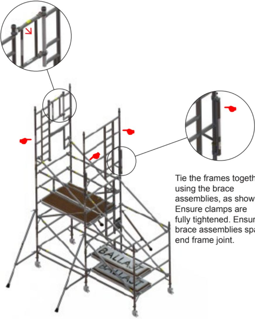
Tie the frames together using the brace assemblies, as shown. Ensure clamps are fully tightened. Ensure brace assemblies span end frame joint.
