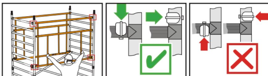
Ensure horizontal braces and guardrails are fitted correctly.
