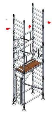
Fit one 1.3m trapdoor deck onto the 8th rung above the platform deck as shown. Ensure wind-locks are engaged.
