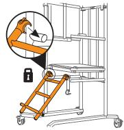
Rotate the ladder down, using the claws as pivots. Locate the bottom of the ladder over the base frame as shown.
