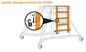
Locate the ladder claws over the spigots on the left and right hand side frame. Ensure the claws are locked.
