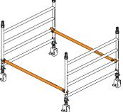
**4** Fit two additional end frames and ensure the frame interlock clips are engaged.
