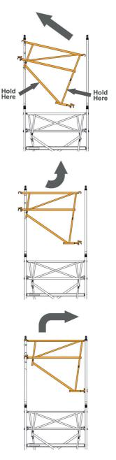
**5.4** Place AGR onto rungs of both end frames, ensuring both hooks and both claws are correctly positioned as shown. Engage locking handle of lowest claw.
