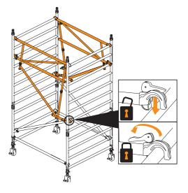
Camlock Advance Guardrail (AGR) Frame Assembly Installation
