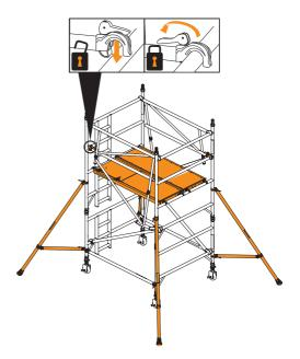
Continue the procedure until the required height is reached, adding additional pairs of end frames, AGR frames and fitting trapdoor/fixed platforms, as shown on previous steps. For every platform level, add AGR frames from the platform below as guardrails (as shown in **Step 5**).
