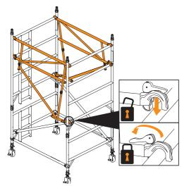
Camlock Advance Guardrail (AGR) Frame Assembly Installation
