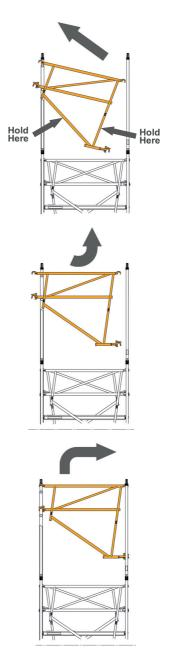
**5.4** Place AGR onto rungs of both end frames, ensuring both hooks and both claws are correctly positioned as shown. Engage locking handle of lowest claw.
