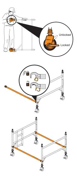
**4** Fit two additional end frames ensuring ladder sections line up and the frame interlock clips are engaged.
