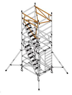
Fit fully hinged trapdoor platform above stairway, as shown. Ensure the trapdoor is positioned with the hinges towards the outside of the tower, as shown.
