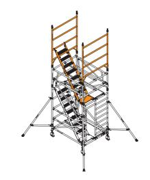
Remove two temporary horizontal braces.
