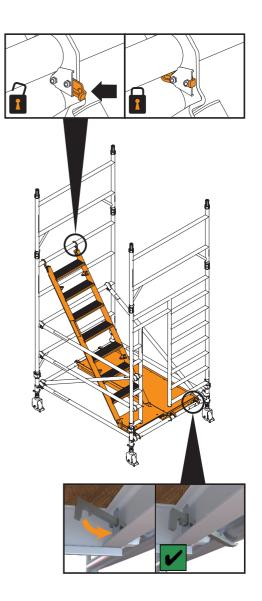
Fit two camlock AGR frames, one on each side of the tower in the positions shown.
