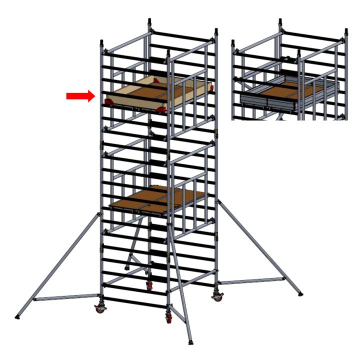
Maximum distance between platforms should not exceed 2.25m. Maximum distance to first platform should not exceed 3.4m
