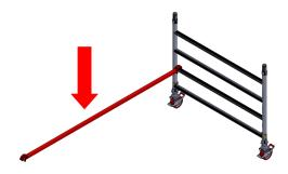
Position the frame as shown. Connect the other end of the horizontal brace to the second end frame. Now connect the frames using a second horizontal brace on the opposite side, attach inside of the rung frame just above the second rung, claws facing outwards, this will square the tower.
