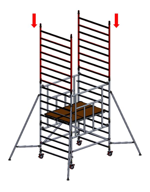
7. Fit a AGR on each side of the tower. The bottom of the AGR must be fitted to the 2nd rung of the 8 rung sides, as shown. The AGR should be placed up against the end frame verticals.
