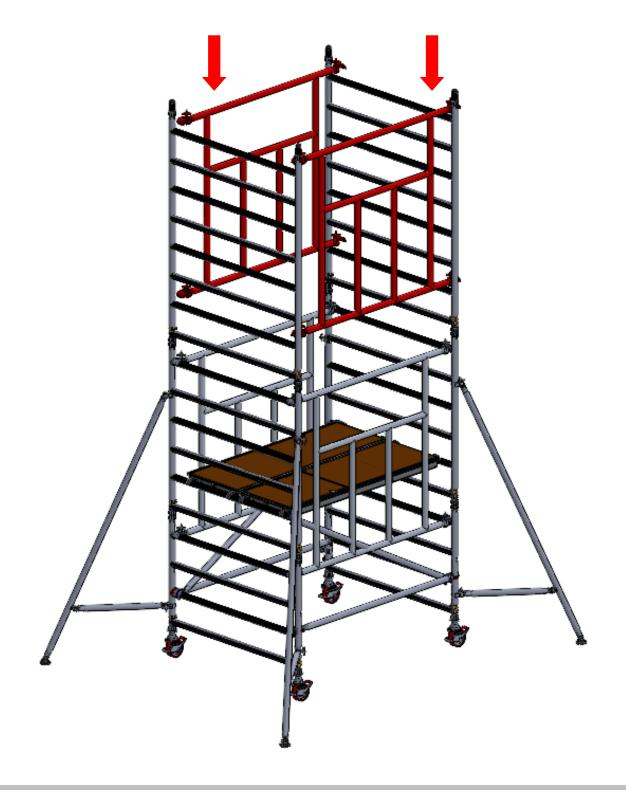
Place a trap door platform and a fixed platform on the 4th rung of the 8 rung frame, ensure the trap door platform is on the ladder side of the structure. LOCK WIND LOCKS.(Refer to Page 9)
