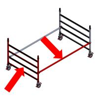
Insert 6 rung frames to correspond with the 4 rung frames (fig. 3) and lock the locking clips (refer to page 9).
