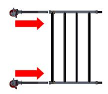
$\label{eq:2.2} Attach one horizontal brace to the second rung of the end \\ \textbf{2.} \qquad \text{frame, claws facing downwards.}$
