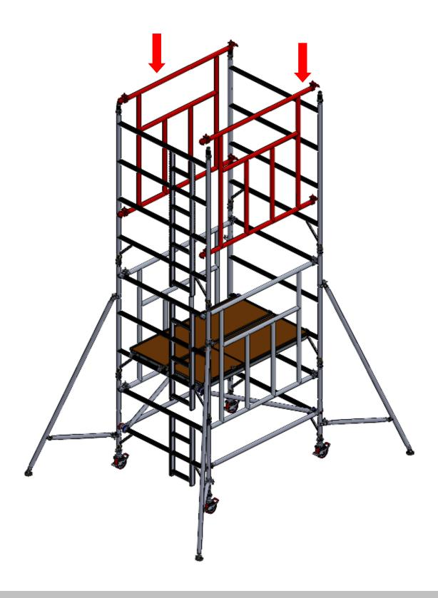
Place a trap door platform and a fixed platform on the 2nd rung of the 4 rung frame, ensure the trap door platform is on the ladder side of the structure.
