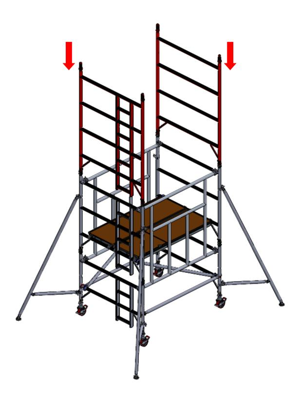
7. Fit a AGR on each side of the tower. The bottom of the AGR must be fitted to the 1st rung of the 4 rung sides, as shown. The AGR should be placed up against the end frame verticals.
