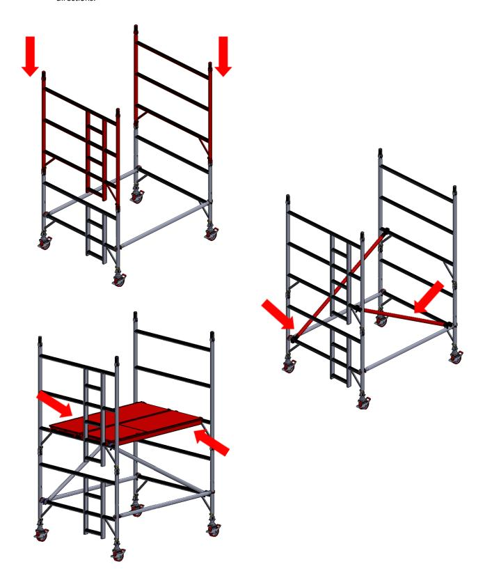
Attach stabilisers as required for working height (see table page 20).
