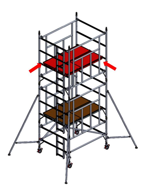
9. Fit toe boards to all working platforms either folding alumnium or toeboard clips and planks. (see instructions on page 9)
