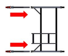
$\label{eq:2.2} Attach one horizontal brace to the bottom rung of the span} \\ \textbf{2.} \quad \text{frame, claws facing downwards.}$
