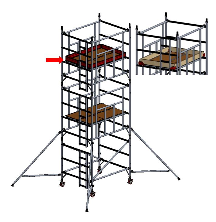
Maximum distance between platforms should not exceed 2.25m. Maximum distance to first platform should not exceed 3.4m
