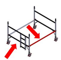
Attach one horizontal brace to the bottom rung of the span frame, claws facing downwards.
