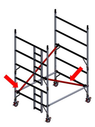
Fit a AGR on each side of the tower. The bottom of the AGR must be fitted to the 2nd rung of the tower, as shown. The AGR should be placed up against the end frame verticals.
