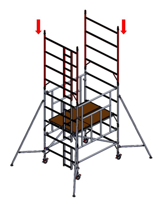
Fit a AGR on each side of the tower. The bottom of the AGR must be fitted to the 1st rung of the 4 rung sides, as shown. The AGR should be placed up against the end frame verticals. Make sure bottom AGRs are locked before you climb tower. (refer to page 9)
