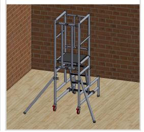
3. Side elevation against a wall. Position 1 stabilisers at 90° from the Podium, and 1 parallel
