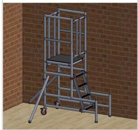
5. In open area, working over sides or overhead, put stabilisers at 90° from body as
