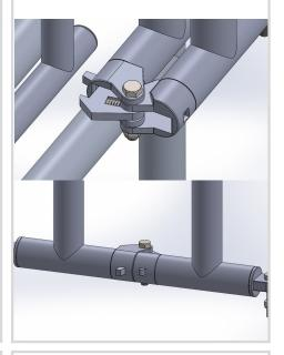
4. Push ladder hooks onto lowest rung between the guides until it locks. Now
