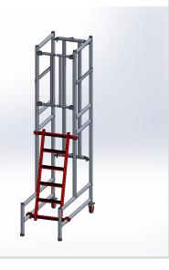
5. Hook on platform at chosen height and turn wind lock to closed position.
