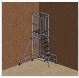
4. In open area, working at rear or overhead, put stabilisers at 45° from body as shown in
