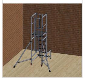
5. In open area, working over sides or overhead, put stabilisers at 90° from body as
