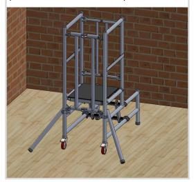
3. Side elevation against a wall. Position 1 stabilisers at 90° from the Podium, and 1 parallel
