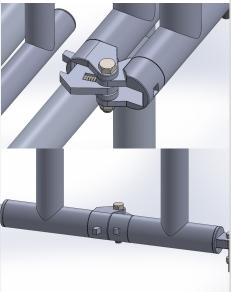
4. Push ladder hooks onto lowest rung between the guides until it locks. Now
